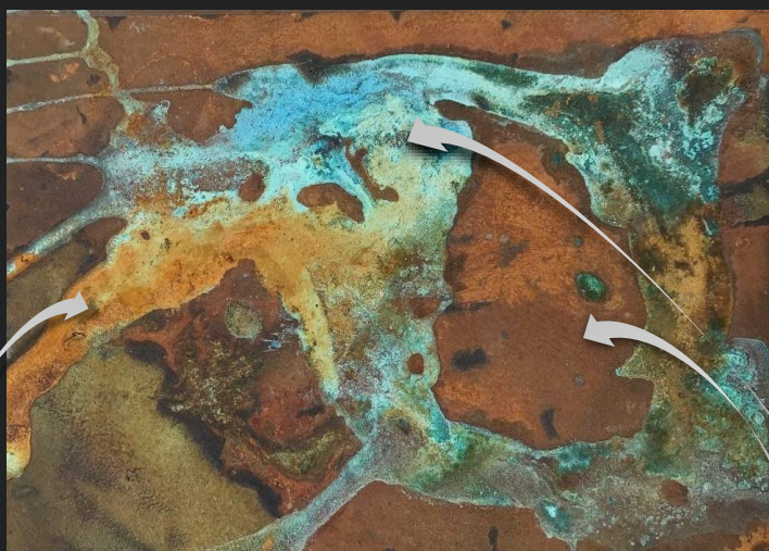
OXIMETAL + RED ACTIVATOR + BLUE NORDIC ACTIVATOR (APPLIED ON FRESH RED ACTIVATOR)
