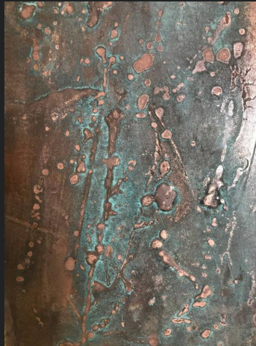
COPPER + NORDIC BLUE ACTIVATOR (WITH PARTIAL FINAL POLISHING)
